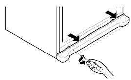
2. Turn the leveling leg clockwise to raise that side of the refrigerator or counterclockwise to lower it. It may take several turns of the leveling leg to adjust the tilt of the refrigerator.
